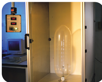
Burst test for safety assurance.
