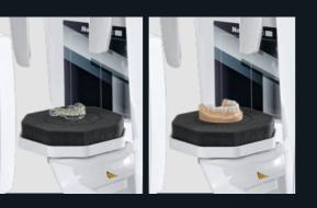
A specific protocol allows for tomographic scans of radiological templates, prostheses, models or impressions after they have been positioned on a special support.
