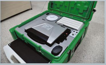
All of the essential parts of the DIARM MW are in a waterproof, shock resistant plastic case. This case is equipped with wheels for transportation, a retractable handle, a pressure valve and hand-carry handle. The transportable case also allows for travel across long distances and quick setup under field conditions.
