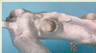
Insert the pre-fabricated housing and bond.
