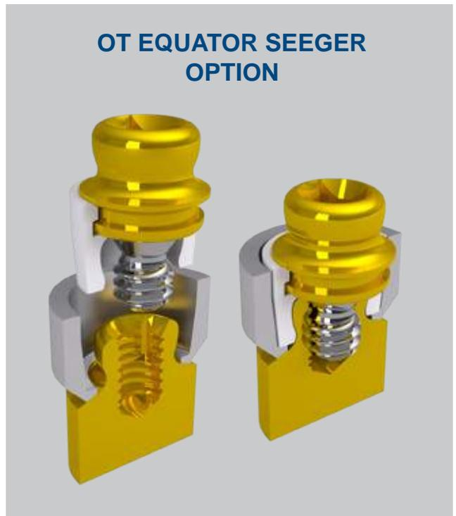
The purpose of the OT Equator “seeger” system is to create a passive connection for implant supported bars. The elastic seeger will correct small imperfections created by the chairside impression technique or laboratory casting process. This reduces the risk of the implant bar to not seat passively.
