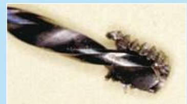
BROKEN SCREW BEING REMOVED
