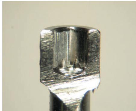
Hexagonal connecting screw 1.26 mm
