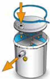
Lead the supply tube into the highest chamber.
