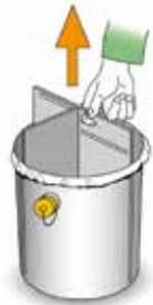
In cleaning release the screw on the drain and unscrew the locking lid. Skim the standing water and pull out the input.
