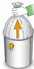
Tie the foil collector under the drain opening and remove it.
