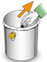
Remove the pipe-fitting from the drain.
